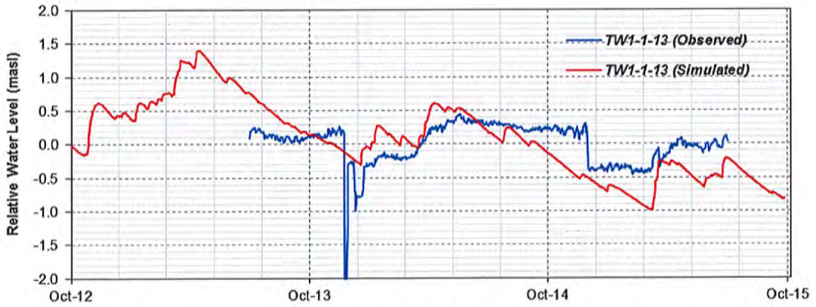
Figure 4.22: Simulated and observed heads at municipal test hole TW-1-13.
